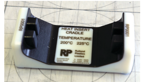
Figure 4: One-piece fixture is printed in a single operation.
