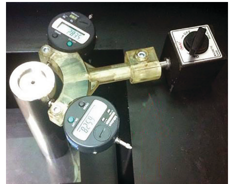
Figure 15: PolyJet 3D printed calibration fixture.
