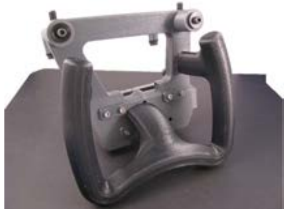
This redesigned FDM tool consolidates most components.
